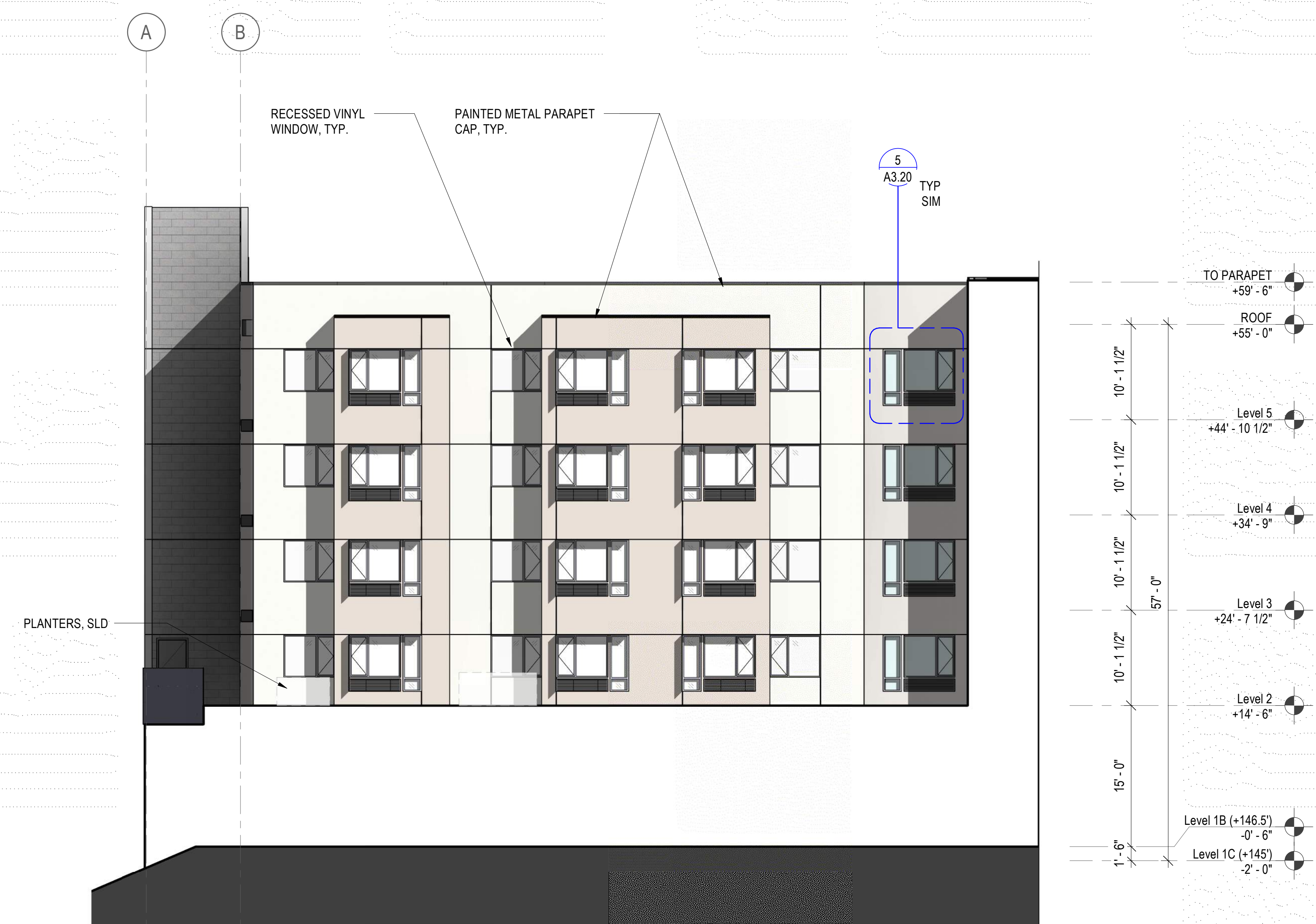
ELEVATION COURTYARD - SOUTH 1/8" = 1'-0" 1
