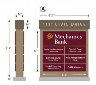
D/F illuminated, 1111 Civic Plaza: ½" Push Thrus Tenant panels, Individual 3D panels with ½" Push Thrus Opaque Aluminum Backgrounds, Textured top cap and structure Mech Bank Panel: 1' 10" x 5' 6", 6.5" letter B Owner/Tenant Panels: 11.75" x 2' 8.5", 7" max letter ht 28" x 84" concrete pad all around base, 6" above grade
