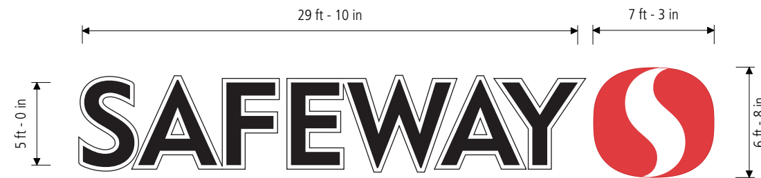
Sign A | Halo Illuminated Reverse Pan Letters w/ Backer Panel. Face Illuminated Logo Scale 1/8"=1'-0" SAF-60-LOCK-LED Sign Area 197.5 SqFt
