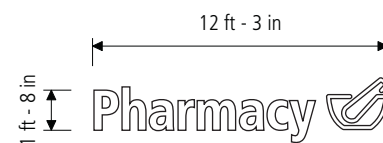
Sign D | Halo Illuminated Reverse Pan Letters Scale 1/8"=1'-0" SAF-20-PHRMICY-LED Sign Area 21 SqFt
