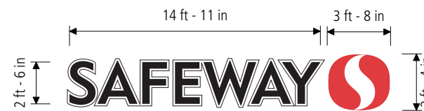
Sign B | Halo Illuminated Reverse Pan Letters w/ Backer Panel. Face Illuminated Logo Scale 1/8"=1'-0" SAF-30-LOCK-LED Sign Area 49.5 SqFt
