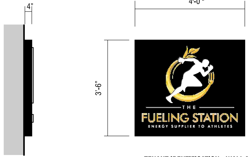
H5 TENANT IDENTIFICATION - WALL MOUNT - FUELING STATION
