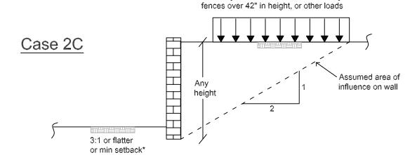
Surcharge from vehicle, tiered retaining walls,
