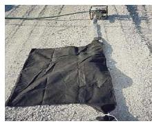
typically flow at the fastest rate with clay flowing the slowest. Clay can also bind over the fabric in some instances blocking flow entirely.
